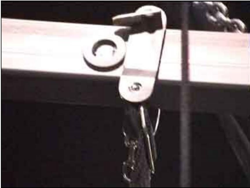
Fig 4.5-11 Attach tilting straps to the grid using the smaller sword pin (On a special fitting that forms part of the strap assembly)
