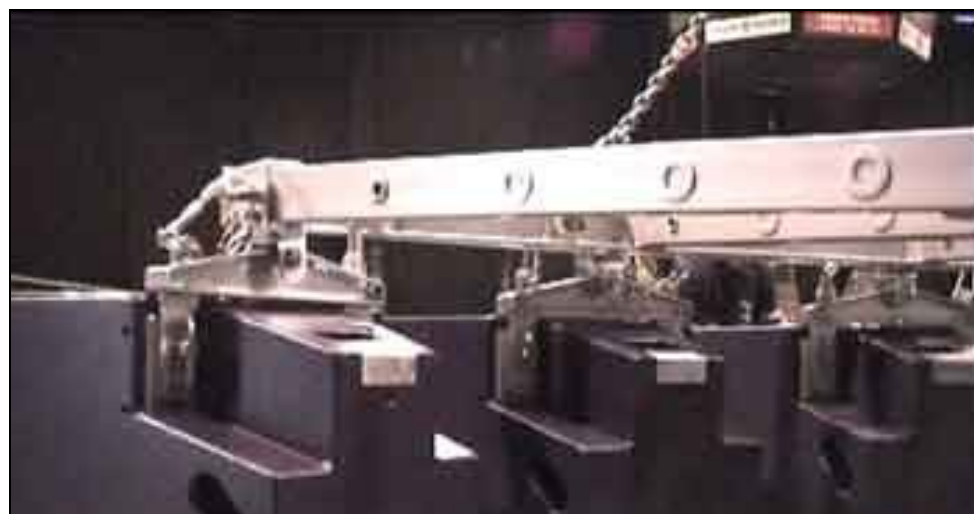
Fig 4.5-10 The toggle pin mated with CH5 column hanger - and repeated with each enclosure on the top row.
