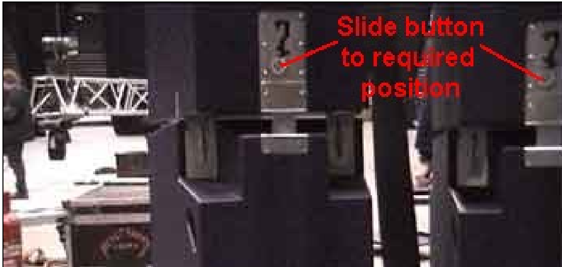
Fig 4.5-18 The 'Biscomatic' auto spacer must be set to achieve the required vertical splay angle between enclosures
