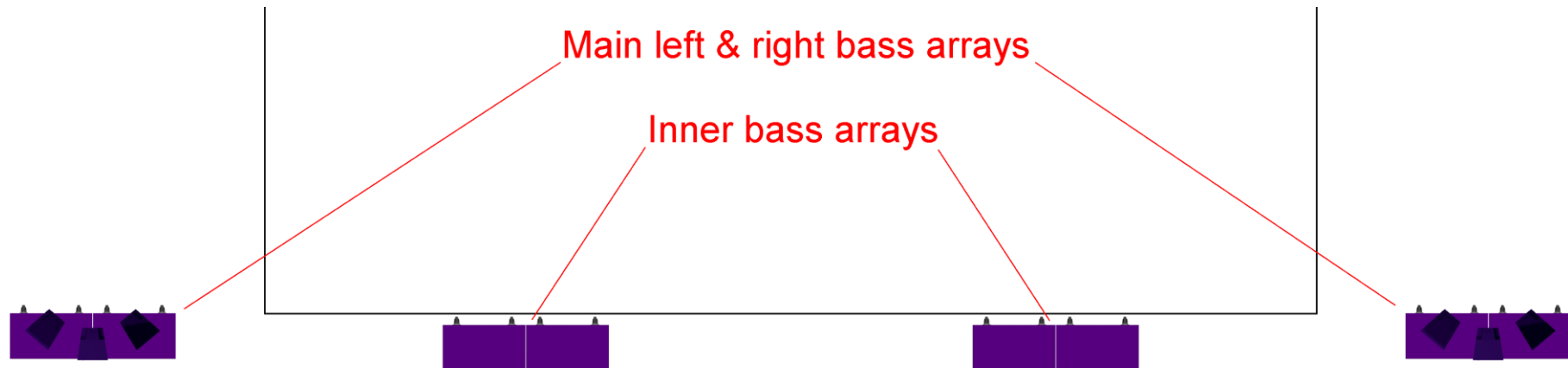
Fig 5.3-8 Inner bass arrays (They also create handy locations for front fills)
