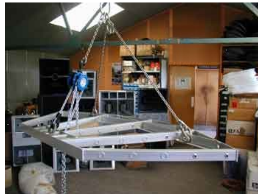
Fig 4.5-1 Grid spokes give the optimum horizontal splay angle (20 degrees for Resolution 5, 40 degrees for Resolution 4)
