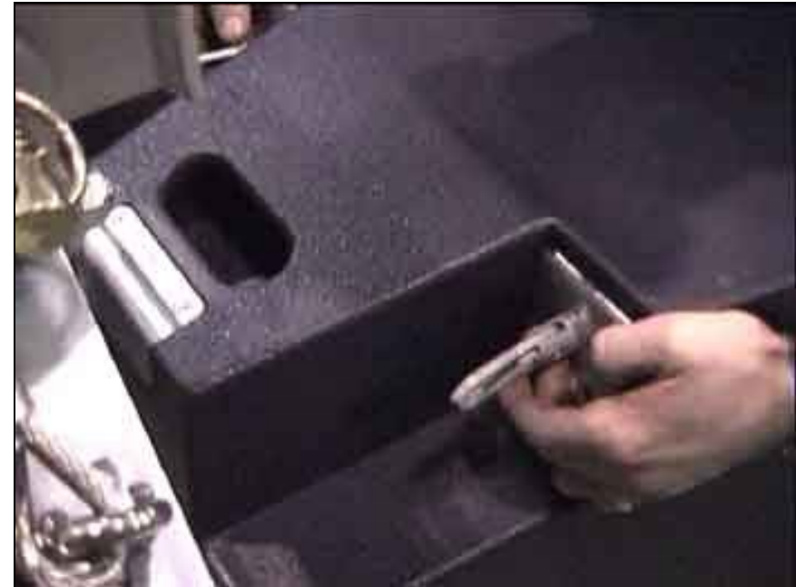
Fig 4.5-7 Antiluce toggle pins on the enclosures ready to go...
