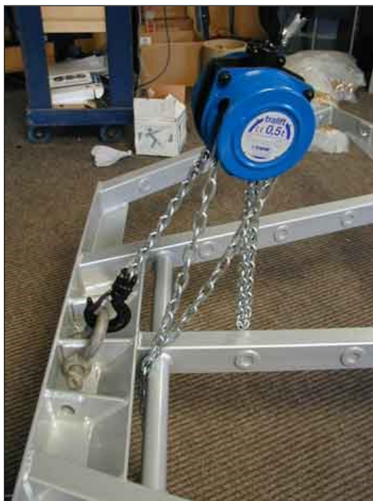
< Fig 4.5-2 Rear view of the grid with hand chain hoist attached via an SH325 bow shackle
